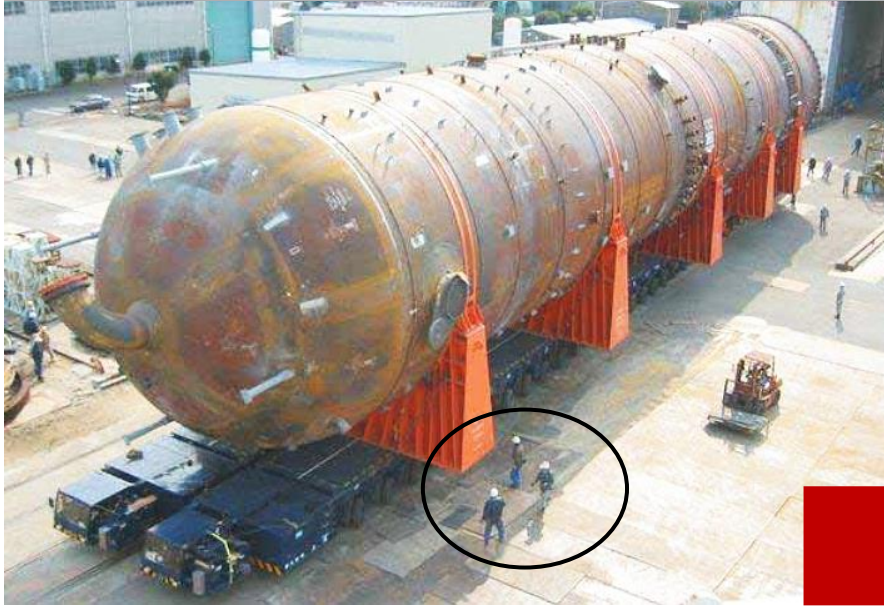
Conventional Fischer-Tropsch reactor
